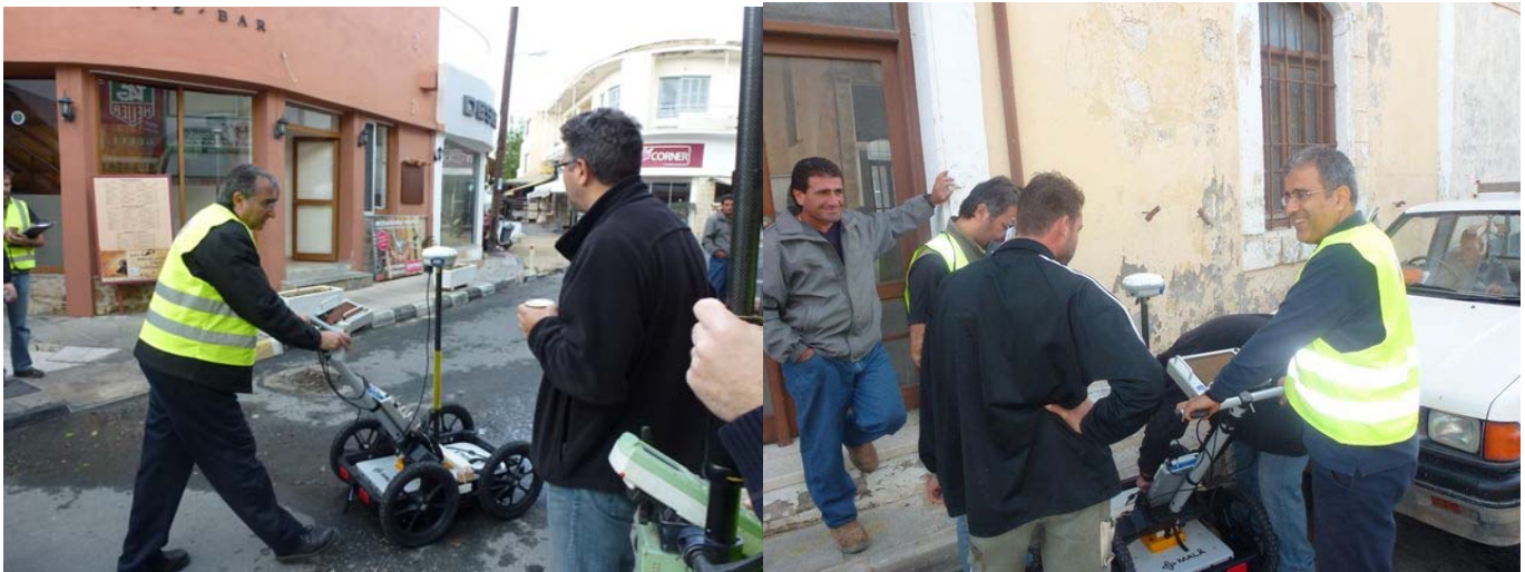
Figure 2 a & b - Geo-radar Scanning of the Paphos water utility network
