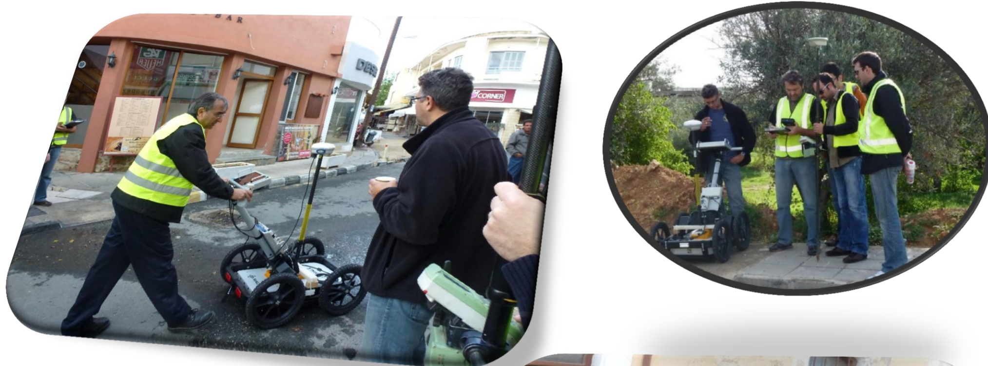
Figure 1.a & b Geo-radar Scanning of the Paphos water utility network
